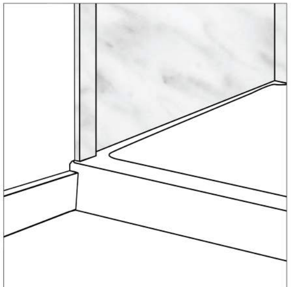
Vertical trims installed on top of shower base
