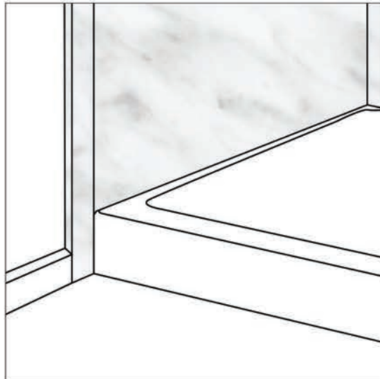
Vertical trims installed outside shower base
